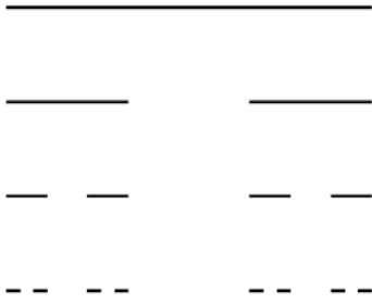
Fig. 20. The triadic Cantor set is created by repeatedly deleting the open middle thirds of a set of line segments. One starts by deleting the middle third from the interval [0,1] , leaving two line segments. Next, the middle third of each of the remaining segments is deleted. This process is continued ad infinitum. The Cantor set contains all points that are not deleted at any step in this infinite process.
